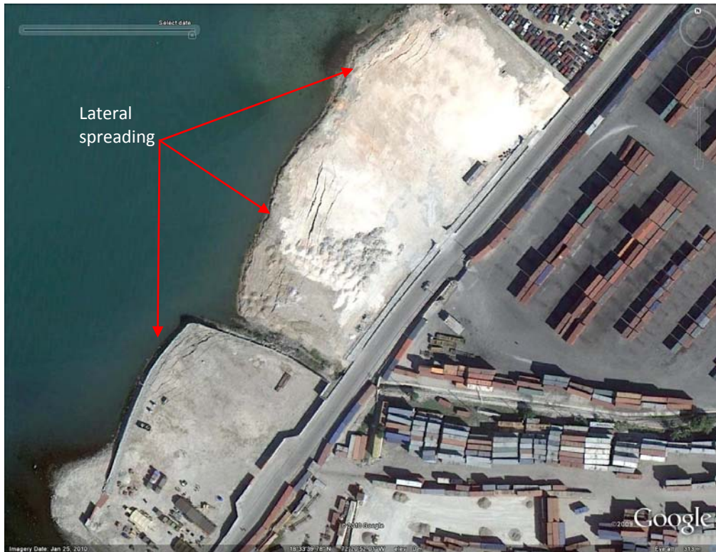
Figure 6.20 Lateral spreading in the storage yards in the northern part of the port facility. Imagery courtesy of Google Earth. ( 18^{\circ}33'40.23''\text{N} 72^{\circ}20'52.33''\text{W} )
