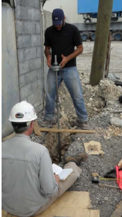
Figure 6.28 Dynamic Cone Penetrometer Test (DCPT). This photograph was taken at the location of DCPT1, facing East. (N18.556681°, W -72.350398°).
