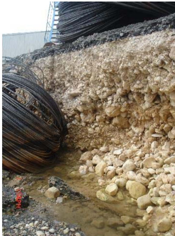
Figure 6.29 Near-surface soil layering at the wharf as observed on the free-face of the lateral spread that collapsed the wharf deck. This picture was taken just south of SASW 1 (refer to Figure 6.26), facing East. (N18.556635°, W 72.350202°).
