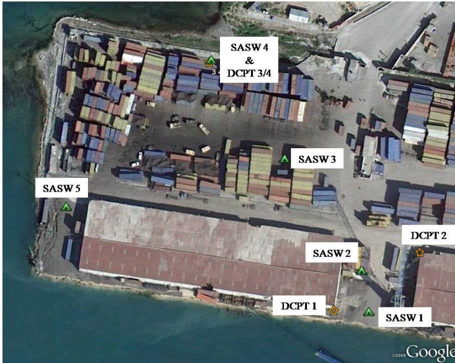
Figure 6.26 Spectral Analysis of Surface Waves (SASW) and Dynamic Cone Penetrometer Test (DCPT) locations at the port in Port-au-Prince Haiti. Imagery courtesy of Google Earth. (Approximate long. and lat. of center of image: 18°33'27.09"N 72°21'03.51"W)
